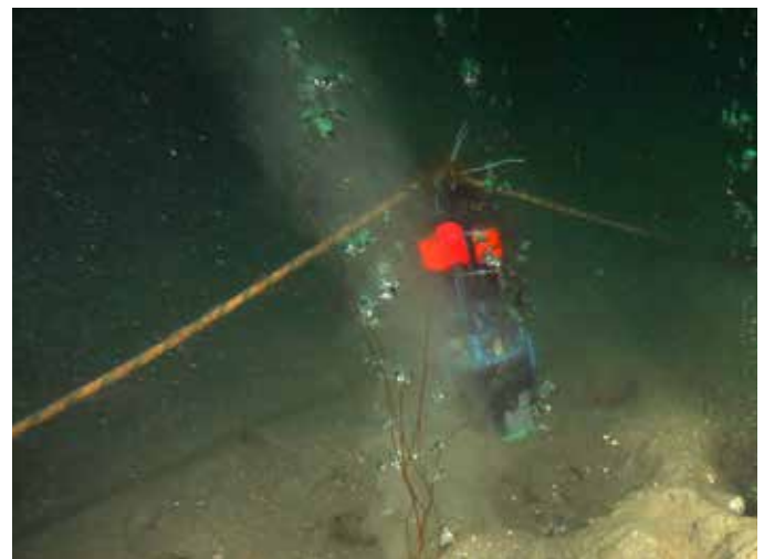
Fig 1: SeaGuard deployed in QICS project at epicenter during a period of CO 2 release. Bubbles were normally only visible during low tide. They dissolve as they rise and are never visible at the surface. Photo courtesy of Henrik Stahl, Zayed University, UAE.
