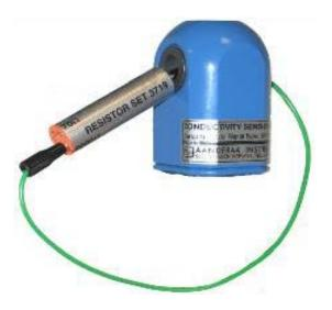
Figure 6-1 Let the resistor wire go through the sensor hole and connect it in the 4 inlets on the other end of the resistor.
