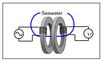
Figure A 4 Transmitter and Receiver Transformer
