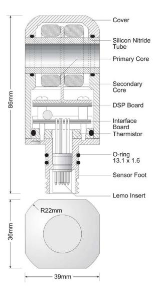
Figure A 2 Drawing of Conductivity Sensor 4319
