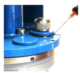
Figure 3-3 Apply Tectyl in the slit between the Sensor and the top end plate. (Example showing tectyl around the electrical terminal).
