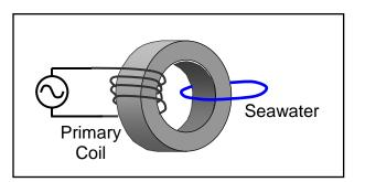
Figure A 3 Transmitter Transformer
