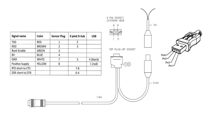
Figure A 6 Set up and configuration cable 3855, for laboratory use.
