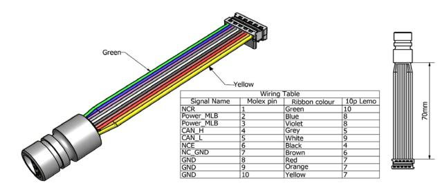
Figure A 11 Drawing Patch Cable 4999, AiCaP
