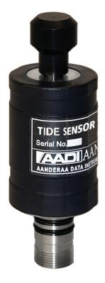
4647/4647R is based on a silicon piezoresistive pressure sensor. The pressure measurements are sampled and temperature compensated by an advanced Digital Signal Processor.
