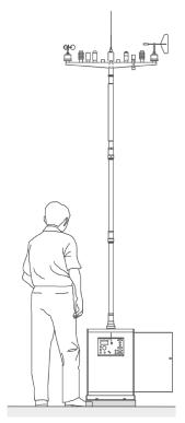
This sensor consists of a light wind vane pivoted on top of a housing. Inside the housing a compass is magnetically coupled to the vane.
