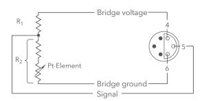
Connecting Cable with Watertight Plugs is available for connecting this sensor to Aanderaa data logging systems. Different lengths, or separate plugs and cables, are available on request. If a connecting cable longer than 150 meters is used, the reading N should be corrected for due to the cable resistance. Add a correction factor of (N - 512) x 0.00011 for each 10 meters of cable used.
