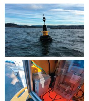
Instrumentation Bay in the top cavity of the Buoy, showing the MOTUS sensor below.
