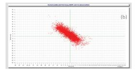
Figure 4: Scatter plots for 3 months of measurements (a) from bottom deployed SeaGuard instruments and (b) from buoy mounted Doppler Current Profiling Sensor.
