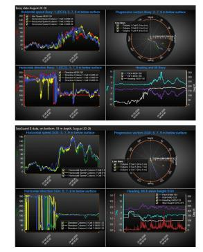
Figure 3: During the first 2.5 days currents agree well in speed, but with about 40-50 deg difference in direction
