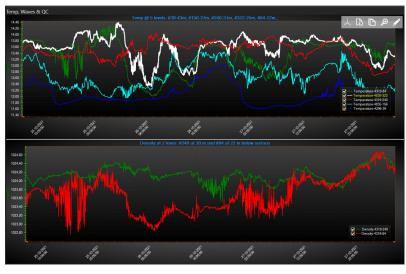
Fig 3: Continuous Temperature (upper graph) and Density (lower graph) measurements with string system. The green line in the density plot is from 35 m and the red from 26 m. Please note the variability and that at occasions, the density is similar at both levels, which indicates that the water is mixed.
