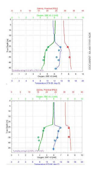
Fig 4: CTD-profiles close to the SeaGuardII mooring before deployment (left) and at the time of recovery (right). The Circles in the left profile indicate the oxygen (green), temperature (blue), and salinity (red) observations by the sensor string connected to the SeaGuardII instrument.
