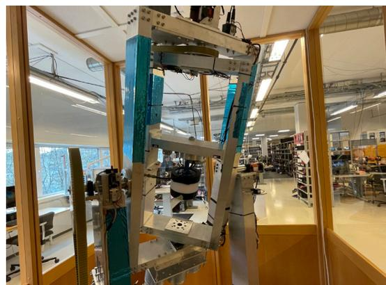
Figure 5: CoTiCa automatic tilt and compass calibration robot inside low magnetic room.
