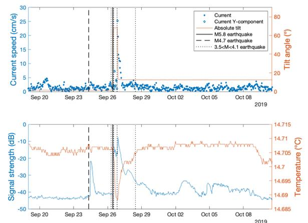
Figure 2. Time series acquired with a **Doppler Current Sensor** (DCS) on a **SeaGuard** during the September 2019 seismicity cluster; (top) current speed and tilt; (bottom) backscatter signal strength and temperature (figure from Henry et al 2022).
