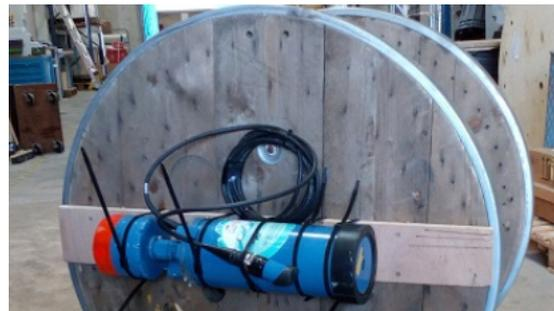
Figure 4: Set up for verifying functioning of inbuilt tilt sensor and compass at high tilt (figure from Henry et al 2022, additional material)
