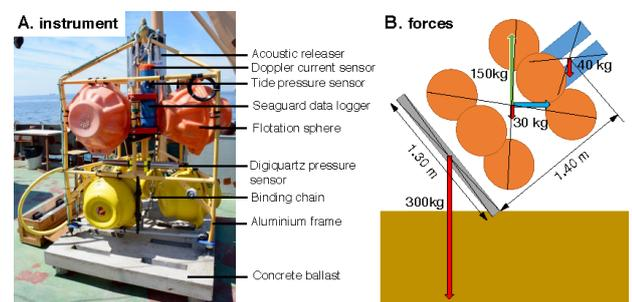
Figure 1. (A) photo of the instrumented frame before deployment. (B) Sketch showing forces applied to the lander after it was tilted over by a turbidity avalanche (figure from Henry et al 2022).
