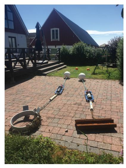
Fig1: Two instrument moorings prepared for deployment. Ballast weight at bottom, chain, acoustic release (thin grey cylinder), instrument, and two floats (white & orange) with lines.
