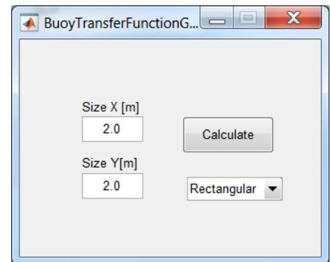
Aanderaa has developed a simple tool that gives an idea on what dampening factors to expect on buoys of different sizes and shape.
