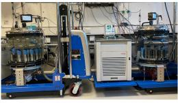
Figure 3: Oxygen multipoint calibration systems at Aanderaa
