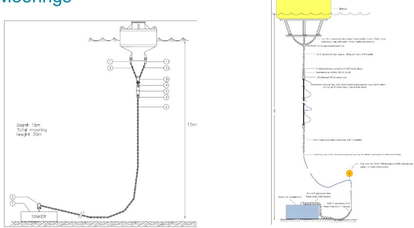
Under 20m, the mooring is constructed with bridle and chain, to stabilize the buoy we usually have around 250-300 kg of mooring in the water (1.75m buoy)
