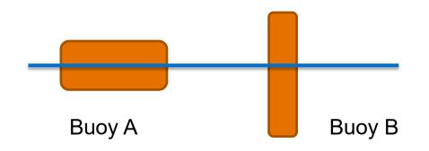
Buoy A will work well for wave measurements, while Buoy B will not
