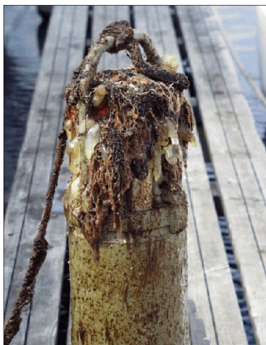
Figure 7-1 Example of fouling on an RCM 9 Mk II with an Oxygen Optode 3830 mounted to it: The Optode was still giving correct readings.
