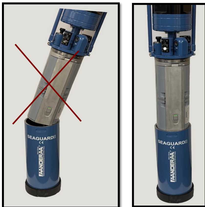
Figure 11-1: Insert Instrument into Pressure Case.
