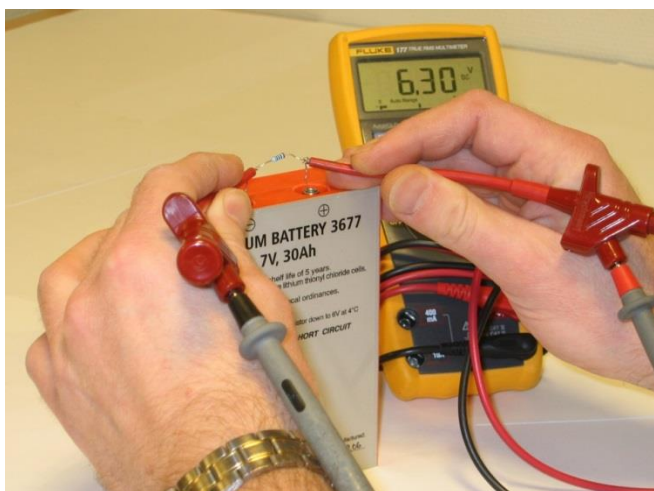
Figure 11-16: Use a 100 \Omega resistor up to 6.3 V to rejuvenate the battery.
