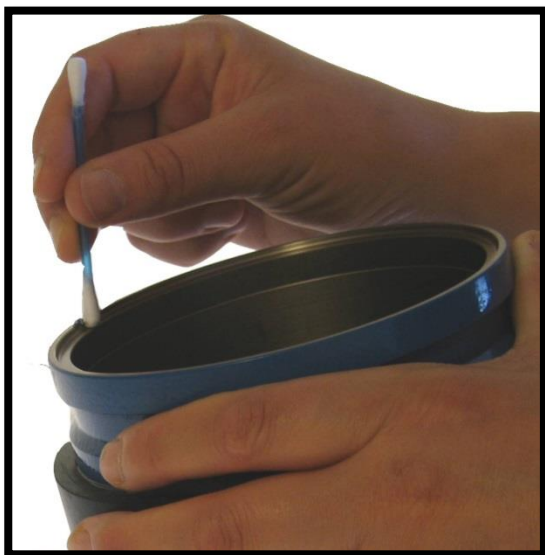
Figure 13-1: Clean o-ring slot using cotton swab
