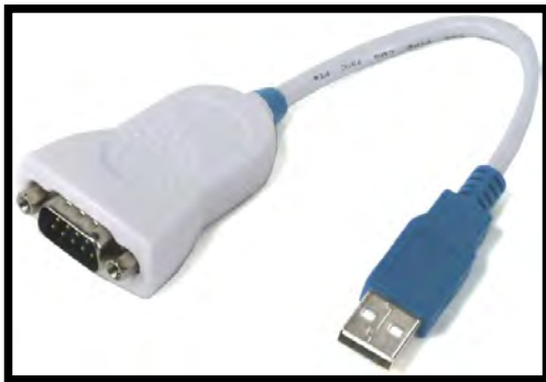
Figure 1-7: Serial to USB converter
