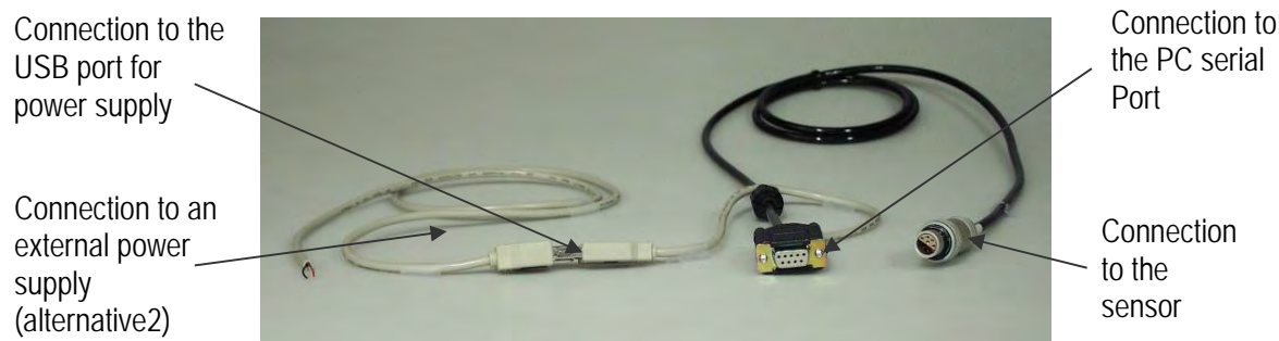
Figure 1-8: Set-up and configuration cable 3855
