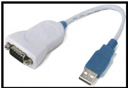
Figure 4-1: FTDI serial-USB adapter
