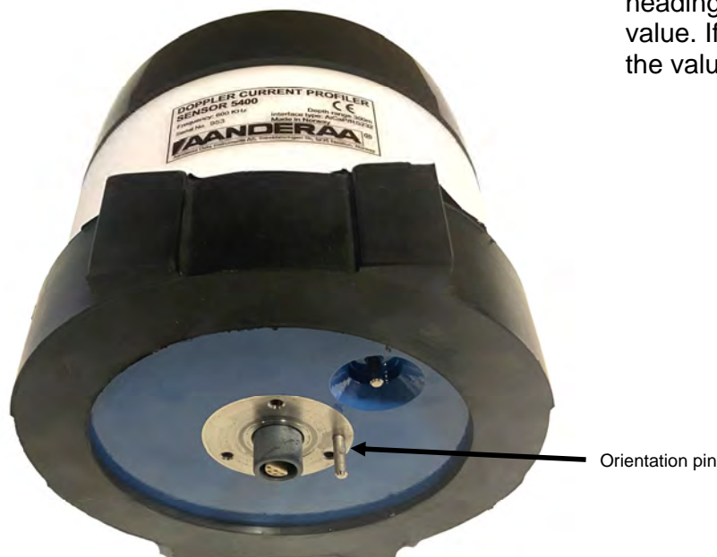
Figure 10-2 Orientation pin and transducers
