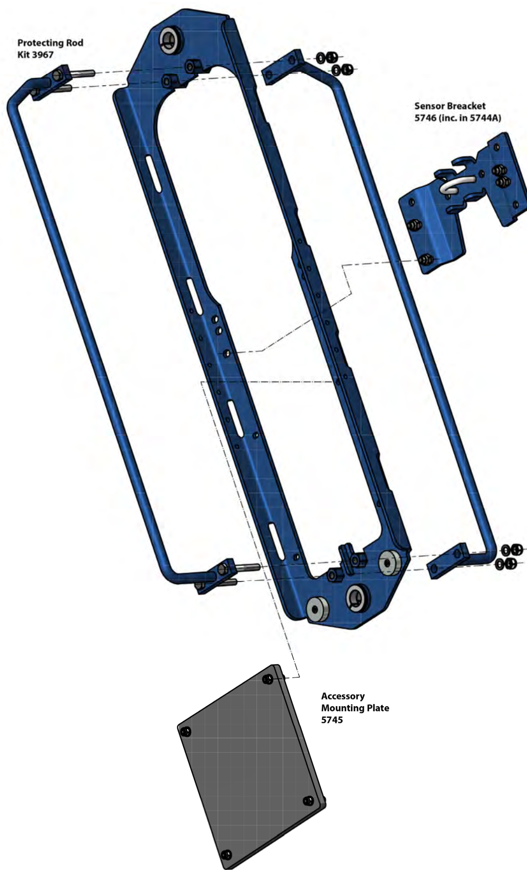
Figure 13-2: Inline mooring frame 5744A
