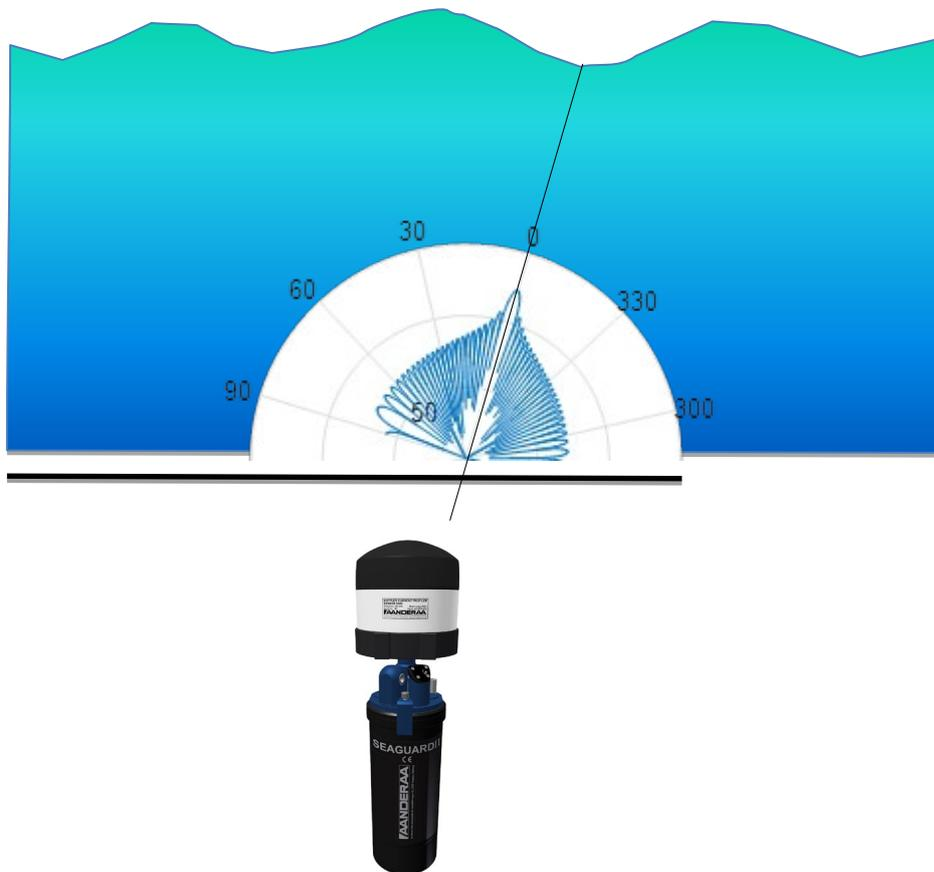
Figure 11-1: Beam geometry and beam pattern concern to avoid surface reflection.
