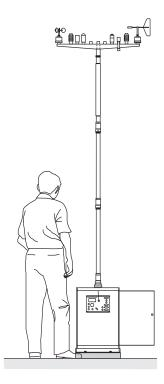
This sensor consists of a light wind vane pivoted on top of a housing. Inside the housing a compass is magnetically coupled to the vane. The sensor can be mounted directly on the sensor arm of the Automatic Weather Station 2700, Data Bouy Sensor Ring on different types of sensor brackets from Aanderaa or on a 25 mm O.D. vertical aluminum tube. When installed on brackets or tubes, the sensor must then be connected to the SmartGuard Datalogger by a separate cable.
