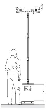
The Wind Speed Sensor 2740 consists of a three cup rotor on top of an aluminium housing. The sensor can be fitted directly onto the Sensor Cross Arms 3415/3435 of an Aanderaa automatic weather station or used separately if a connecting cable is used. The sensor foot will fit onto a 25 mm vertical tube.
