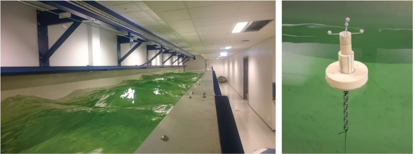
Figure 5: Tank test facility. Validation of the IMU in tank reference system and optical reference system
